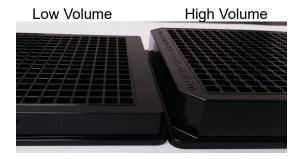
The shape of the wells refers to the shape created by the well walls, not the well-bottom. The most common well shapes are round and square. Round wells are typically found in 6-well to 96-well plates, while square wells are often used in 384-well plates because they provide a larger surface area for the well-bottom. However, round wells are sometimes used in 384-well format to minimize assay volume.
